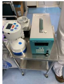
Figure 1: Coriolis Compact air sampler and particle air counter
