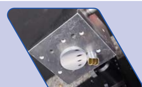
Dual reflector for in-vessel photometry calibration
