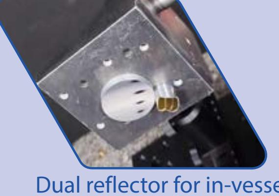
Dual reflector for in-vessel photometry calibration
