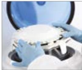
2. Place the holder on the instrument and place tubes on the holder.
