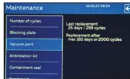
The first indicator shows the number of days since the part was replaced. The second indicator shows the number of cycles performed with the part.
