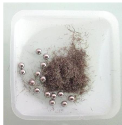
1g of hair after grinding with Precellys (7200 rpm – 3 x 20s (20s of break))
